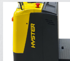
Easy Service Access via Front Cover
