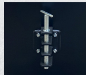
Rear Multi-Position Tow Coupling
