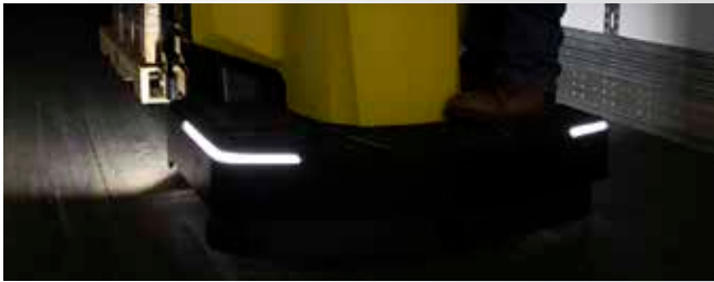
LED platform and trailer lights on the Hyster end rider.
