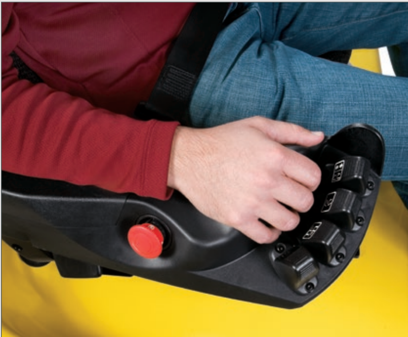
Electro-hydraulic controls with TouchPoint mini-levers
