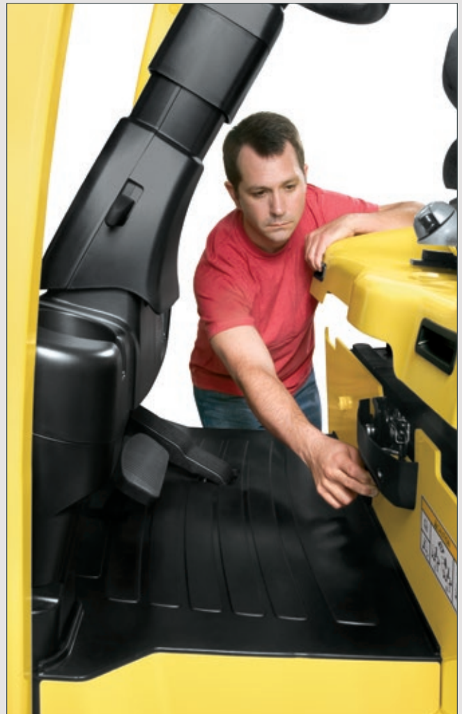
A spring-assisted hood and quick release handle make battery access easier than ever.
