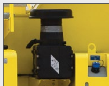
Tier 4 Final integrated pre-cleaner and air filter
