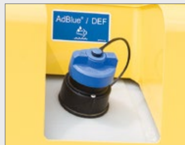
Diesel Exhaust Fluid (DEF) tank
