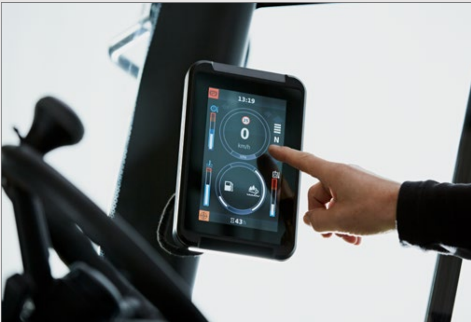
A 7 inch full-color Integrated Performance Display provides truck performance data in one clear screen.
