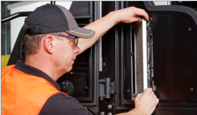
Easy access interior cabin filter
