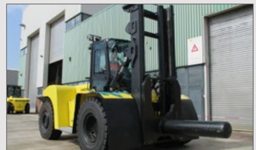
Apron-style sideshift with individual hydraulic fork positioning
