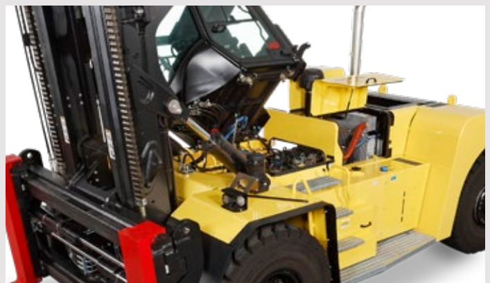
Optional powered cab tilt provides easy access to major hydraulic components
