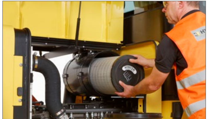
Gull-wings provide easy access for quick service checks
