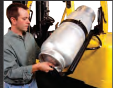
Swing-out drop-down EZXchange bracket
