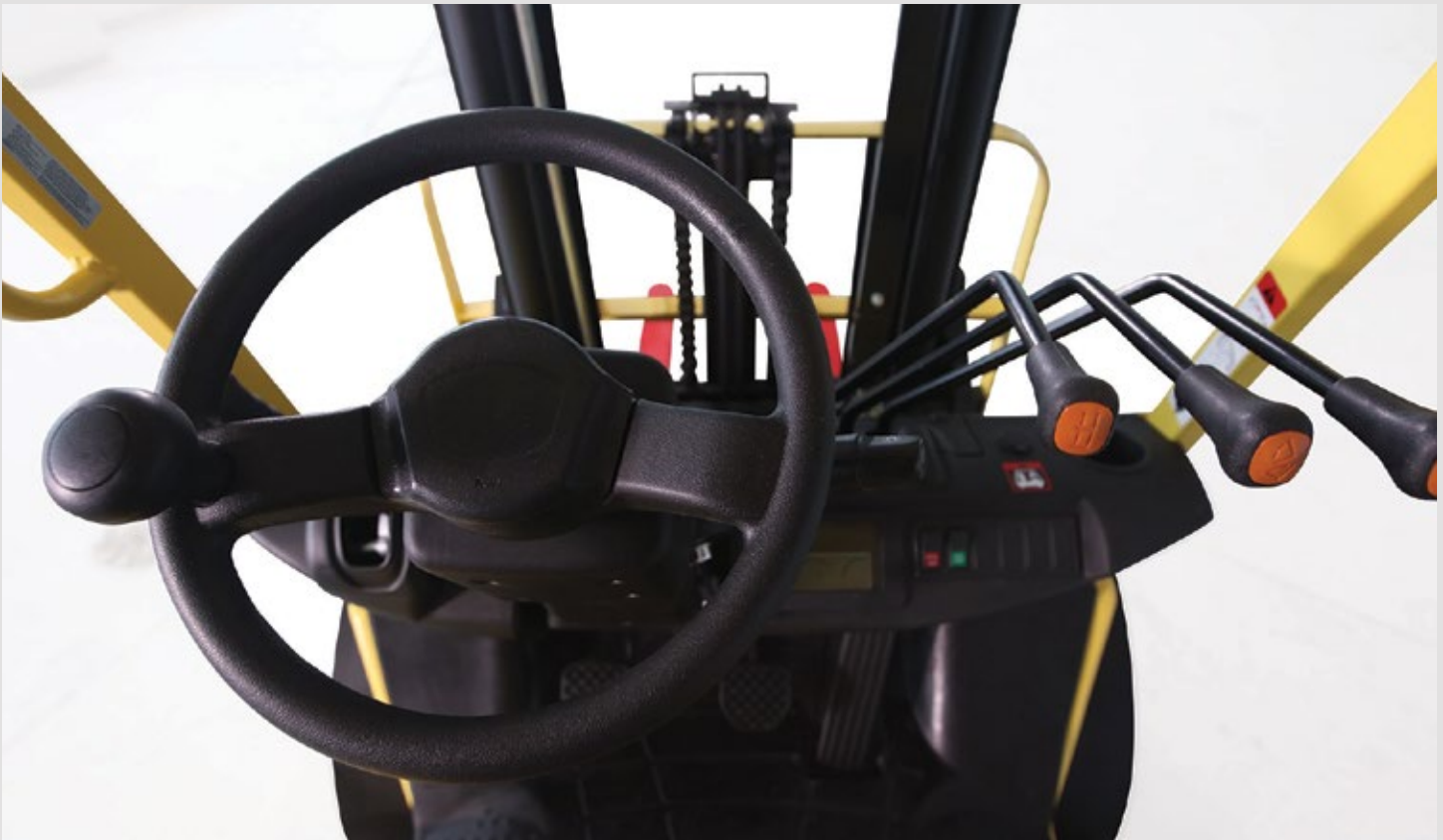
The small, 11.8" diameter steering wheel is easy to manipulate and very responsive. The adjustable steer column affords 8 degrees of adjustment to suit a variety of operators
