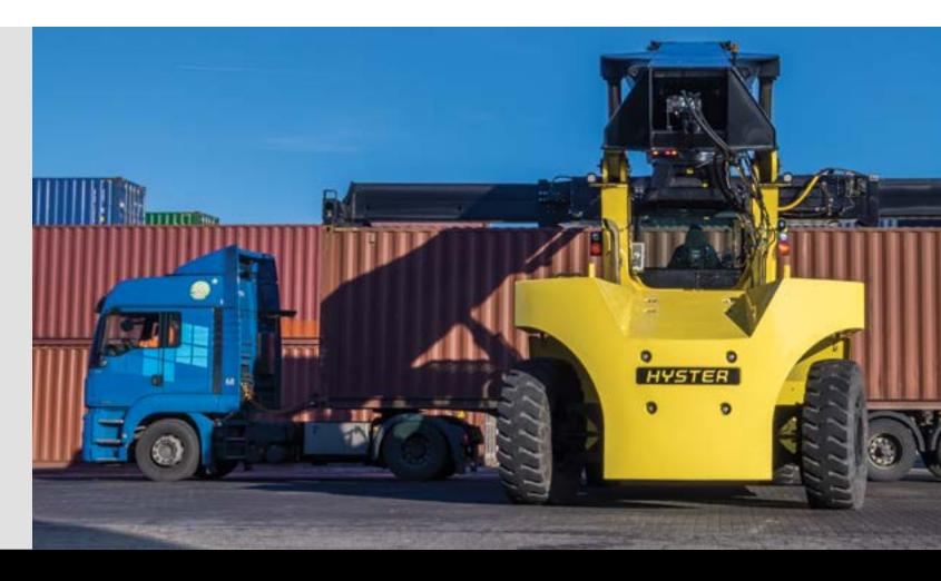
On-demand features help to lower the overall cost of ownership, by increasing component life and reducing service requirements. For example, the cooling fan operates only when required, reducing accessory loads on the powertrain, consuming
