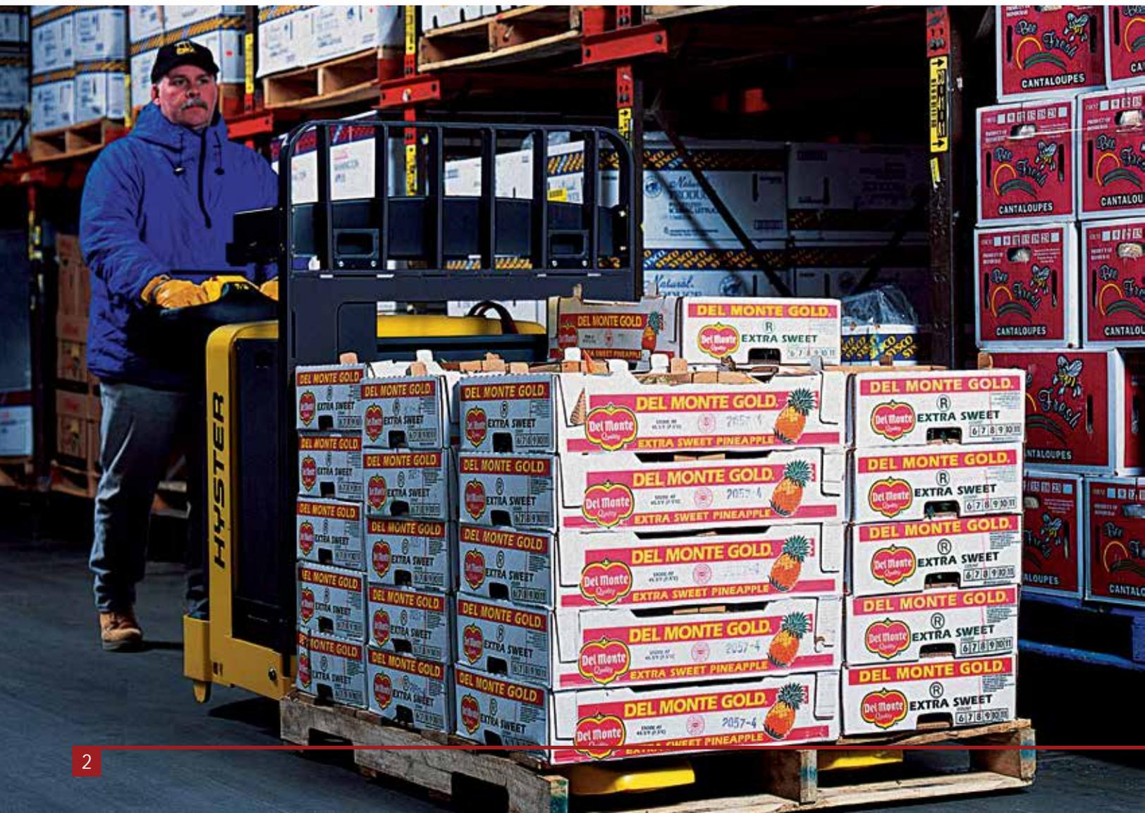
The W80Z truck's bottom-mounted handle conveniently provides you control of all functions with either hand, including the horn. Its angle hand-grips and raised body design provide "when-you-need-it" protection for your fingers and knuckles.
