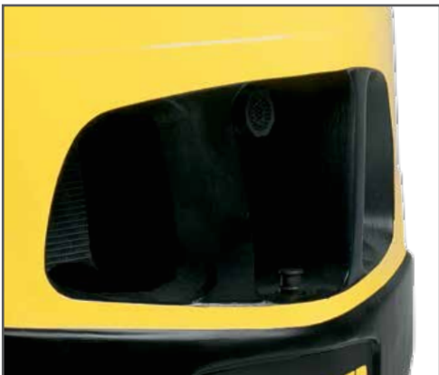
Counterweight tunnel design improves airflow
