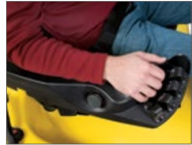
Electro-Hydraulic Controls with TouchPoint Mini-Levers
