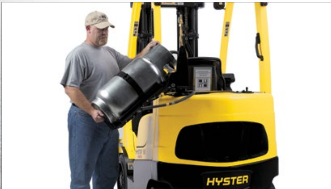
Optional Swing-Out, Drop-Down EZXchange Tank Bracket
