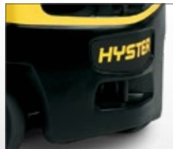
Counterweight tunnel design improves airflow
