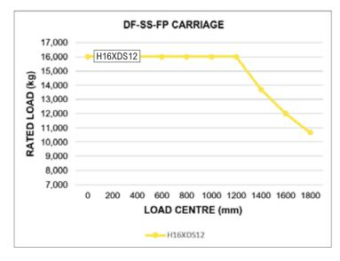
Load centre - distance from front of forks to centre of gravity of load. Rated load - based on vertical mast. Graphs are based on 4594 mm TOF (h3 + s (mm)) lift height
