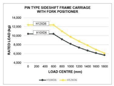
Load centre - distance from front of forks to centre of gravity of load. Rated load - based on vertical mast.
