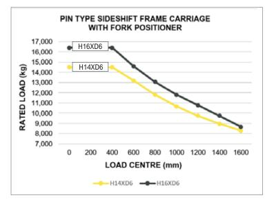
Load centre - distance from front of forks to centre of gravity of load. Rated load - based on vertical mast. Graphs are based on 5000 mm TOF (h3 + s (mm)) lift height. XD6 models are calculated with 1830 mm long forks. Long load centre capacities are for reference only and will require longer forks. Please request actual capacity based on the full configuration.
