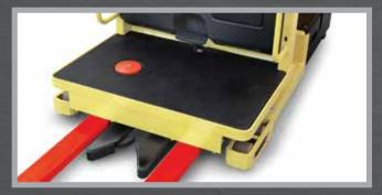
The pallet clamp automatically centers and grips the pallet to allow fast, easy order picking. The foot-operated pedal is easily actuated for quick pallet release. For special pallet handling, we offer a pallet grab with an opening from .5" to 6".
