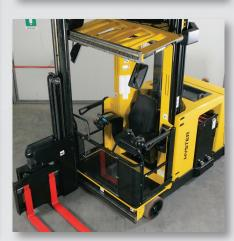
Very narrow aisle warehouses are the solution for many of today's storage and distribution companies who need to reduce costs and increase output. Hyster's latest, range of state-of-the art VNA (Very Narrow Aisle) man-up truck is designed to meet the customer's needs by allowing maximum storage density with narrow aisle widths and maximum operating clearances.
