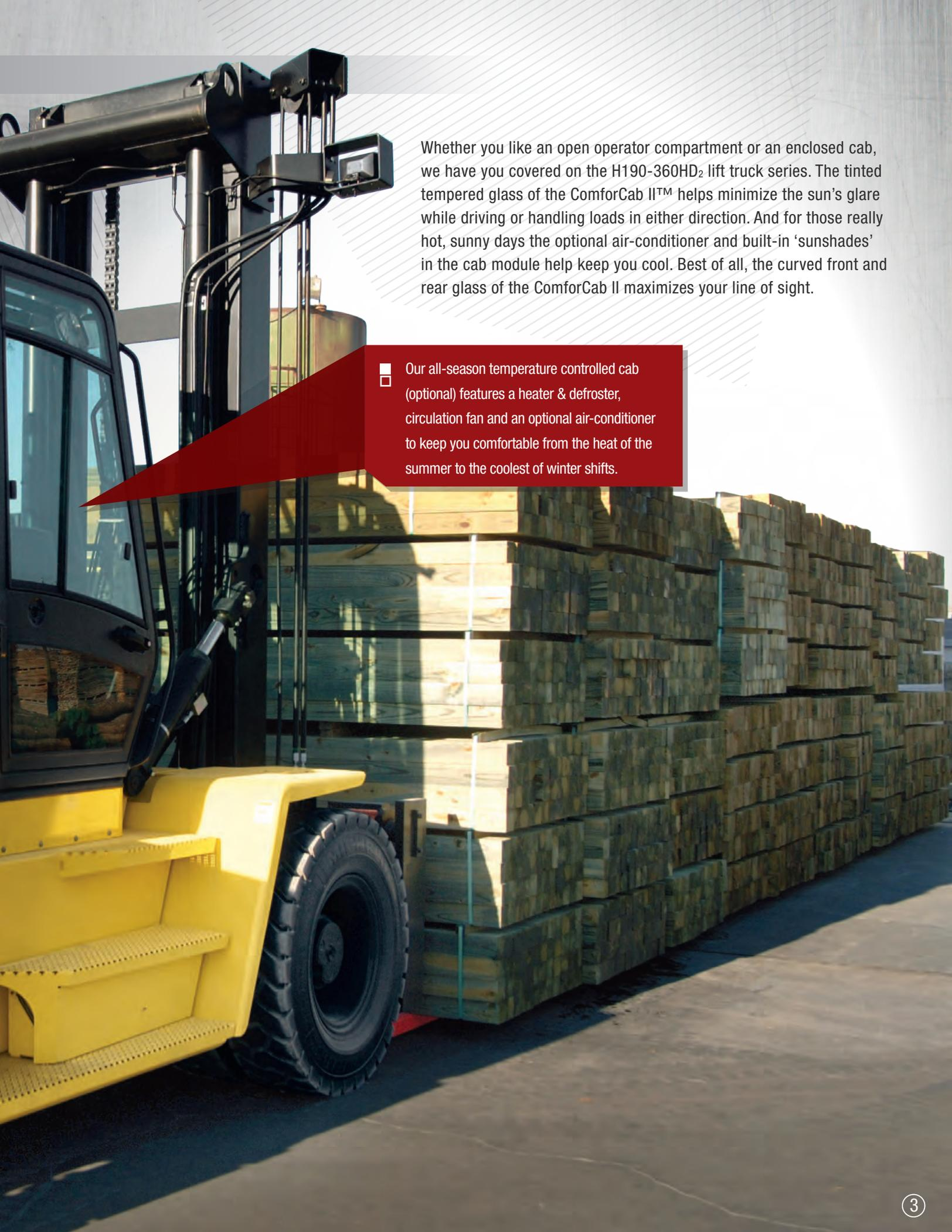
Whether you like an open operator compartment or an enclosed cab, we have you covered on the H190-360HD<sub>2</sub> lift truck series. The tinted tempered glass of the ComforCab II™ helps minimize the sun's glare while driving or handling loads in either direction. And for those really hot, sunny days the optional air-conditioner and built-in 'sunshades' in the cab module help keep you cool. Best of all, the curved front and rear glass of the ComforCab II maximizes your line of sight.
