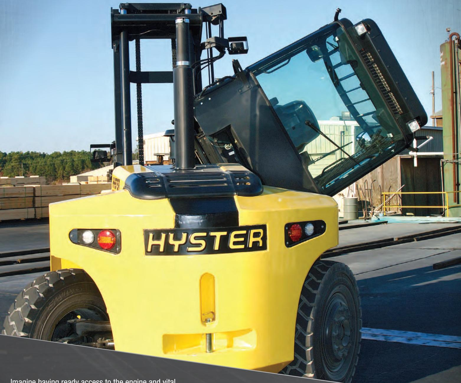
Imagine having ready access to the engine and vital functions of the truck without straining or tying yourself in knots. The answer is the side tilting ComforCab II of the Hyster® H190-360HD<sub>2</sub>. The cab, mounted on 4 rubber isolators pivots over to the right-side of the truck, giving you complete access to all the major components.
