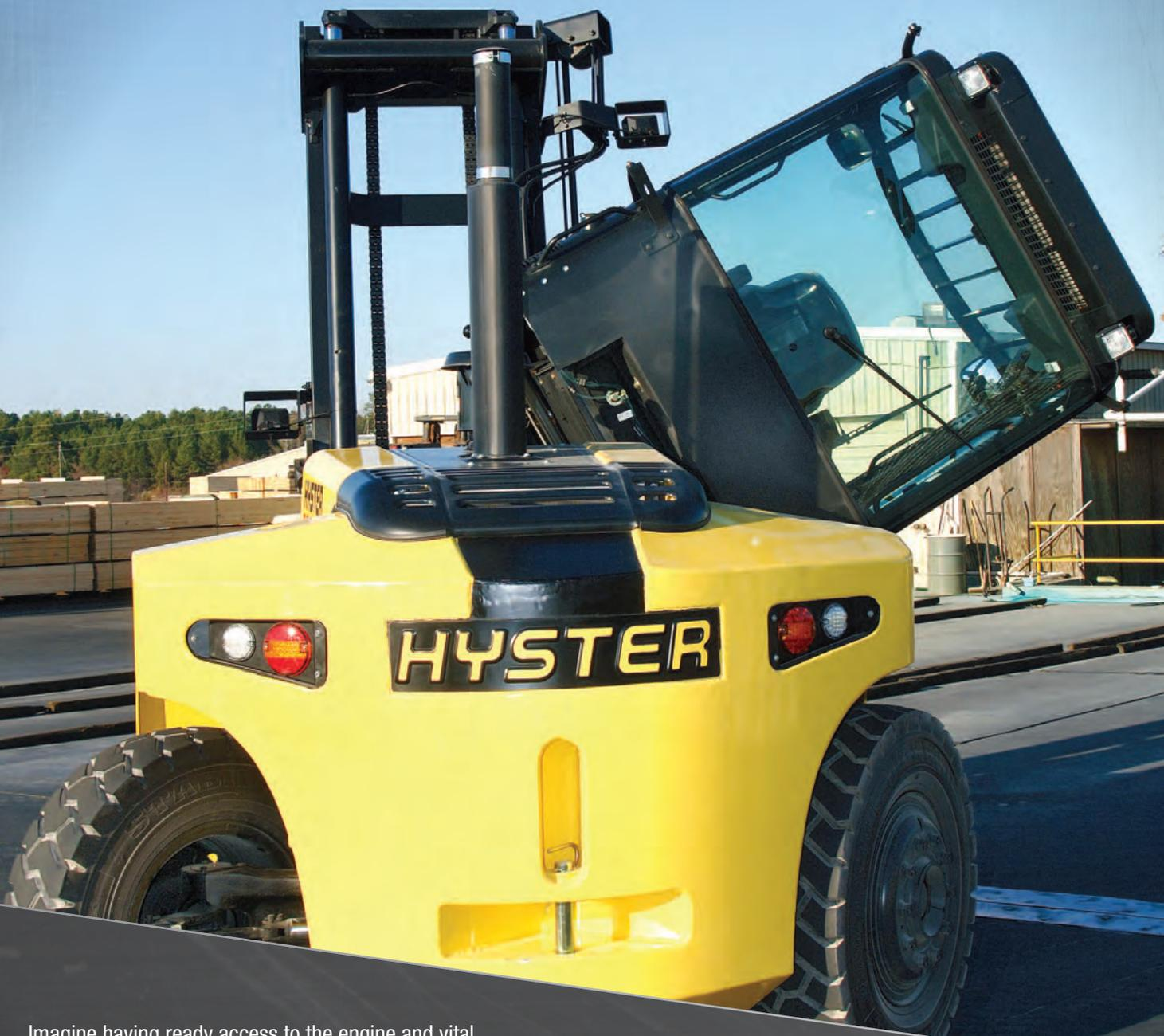
Imagine having ready access to the engine and vital functions of the truck without straining or tying yourself in knots. The answer is the side tilting ComforCab II of the Hyster® H190-360HD<sub>2</sub>. The cab, mounted on 4 rubber isolators pivots over to the right-side of the truck, giving you complete access to all the major components.
