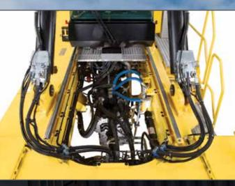
The easily removable top deck plates with quick disconnect latches provides fast access to major components. The CANbus truck and spreader controls enable fast and easy fault diagnosis.
