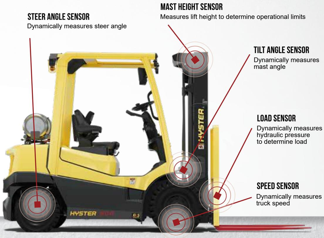
DSS actively monitors five integrated maintenance-free sensors during operation to provide information to the Vehicle System Manager (VSM). The VSM will engage DSS by providing audible and visible alerts from the operator display and limiting truck performance. If telemetry is available, the system will also send an alert to the telemetry portal.
