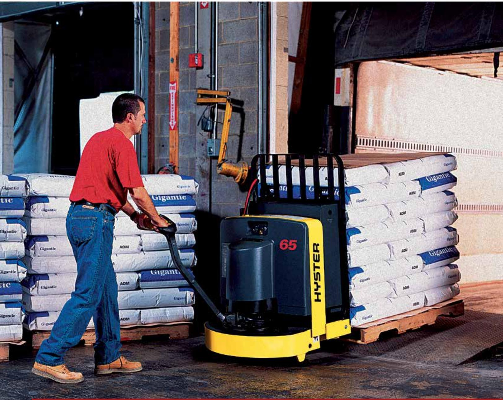
The W65Z truck's bottom-mounted handle conveniently provides you control of all functions with either hand, including the horn. Its angle hand-grips and raised body design provide "when-you-need-it" protection for your fingers and knuckles.
