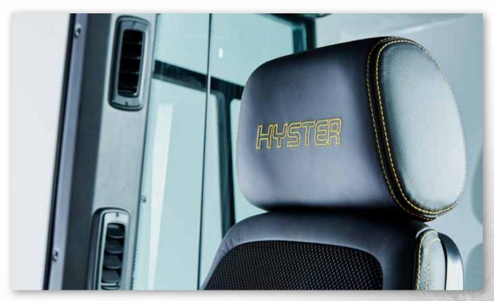
The air conditioning system can be pre-set for automatic climate control, as well as easily adjusted through the Integrated Performance Display or from the panel on the control arm. The unique high and rear louvers provide direct air flow toward the operator.
