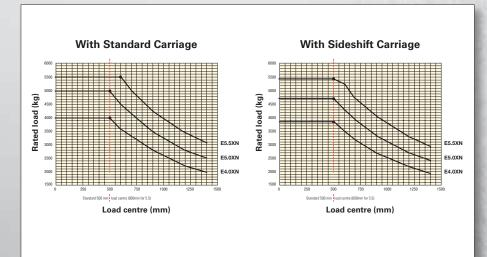
**Load centre:** Distance from front forks to centre of gravity of load. **Rated load:** Based on vertical masts up to 4 600 mm to top of forks.
