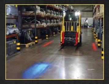
Front and rear blue motion-activated spotlights alert pedestrians that the truck is travelling in a specific direction.
