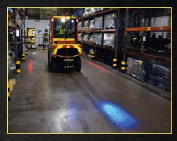
Red zoning lights on either side indicate to pedestrians the required distance that should be kept from the truck when in motion.
