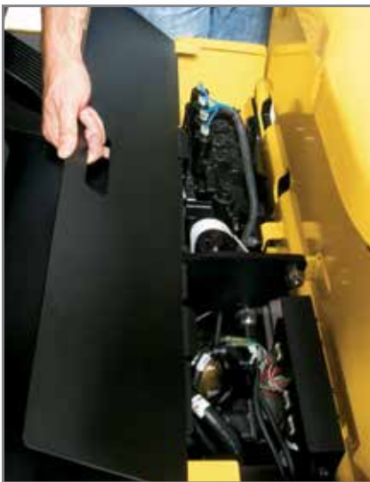
Easy-to-remove floor plates allow full service access for simplified daily maintenance.
