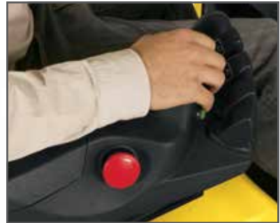
Electro-hydraulic controls with TouchPoint mini-levers
