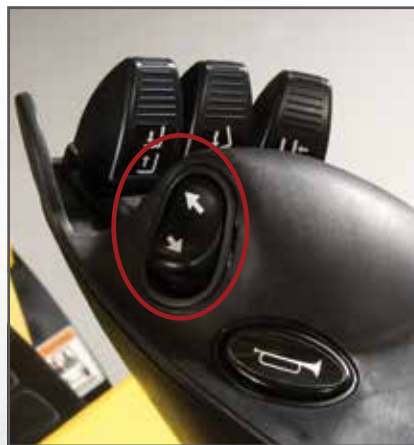
Electro-hydraulic controls with TouchPoint mini-levers
