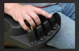
Adjustable armrest that accompanies the optional TouchPoint e-hydraulic control moves with the seat and telescopes forward/vertical in one simple movement to provide greater flexibility in achieving a more custom position.
