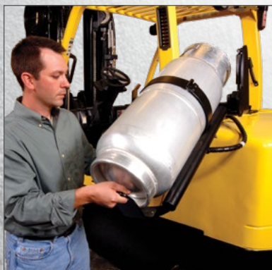
Swing-out EZXchange bracket
