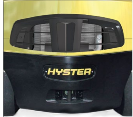
Counterweight venting improves airflow
