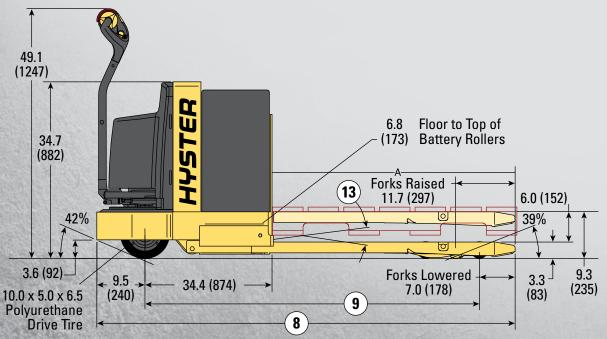
Circled dimensions correspond to the line numbers on the tabulated chart inside the Technical Guide. Dimensions are in inches (millimeters).
