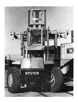
capacity of 62,000 pounds at 48 inch load center. Container handling attachments reduce capacity somewhat, but there's still plenty left to do the job. Here the operator is backing up with the empty attachment high in the air. Note the excellent visibility he enjoys.
