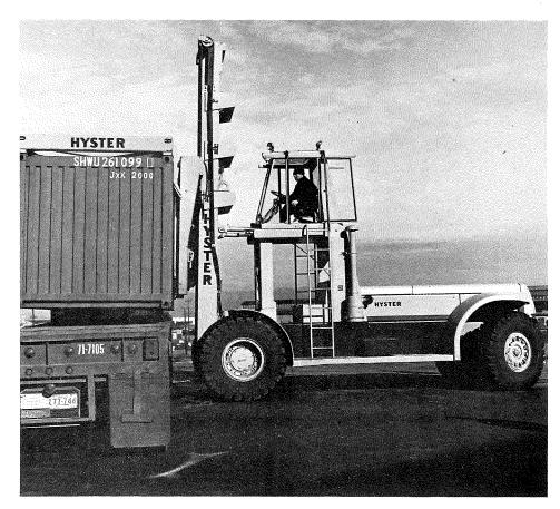
UNLOADING TRUCKS is just one of several tasks performed by the Port of Longview's Hyster Container Handler. Loaded or unloaded; 20 foot or 40 foot containers; dock-side or stacking yard; it makes no difference to the operator of this machine. He can handle any and all situations.
