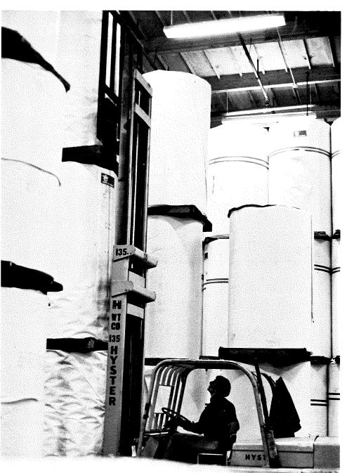
BEST USE OF FLOOR SPACE is achieved by stacking paper rolls three, or even four high, according to size of rolls. Waterway Terminals has been
