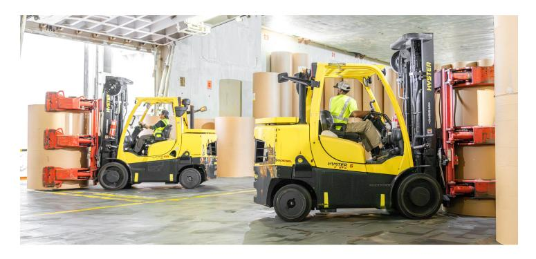
The team recommended replacing the current fleet of high-capacity trucks used in the warehouse with Hyster® Big Trucks, rated at capacities of 23,000 and 36,000 pounds, and a variety of Bolzoni paper-handling attachments. The team also recommended special engineering customizations, including a short wheelbase chassis to enhance maneuverability, a unique lift height mast to maximize facility storage through high stacking and hydraulic refinements to support smooth paper clamp movement.
