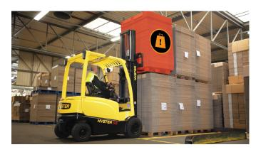
**// OVERLOAD ARREST** to prevent lifting and carrying loads that exceed weight limits
