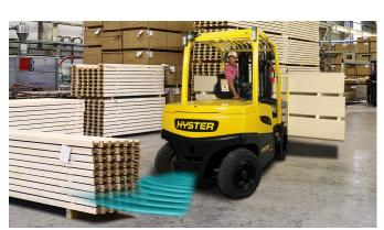
// COLLISION AVOIDANCE ASSIST by noticeably reducing the travel speed when obstacles are detected
