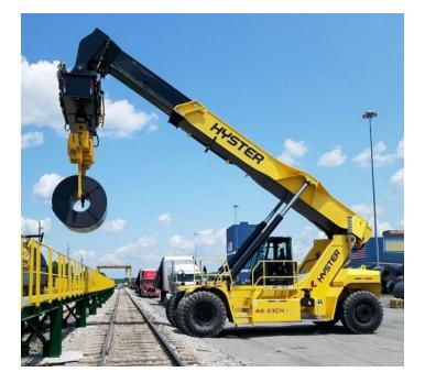
But a reach stacker appropriately equipped for coil handling can safely and effectively execute all of the coil picking, transportation and loading functions handled by fixed or moving cranes, conventional counterbalance lift trucks and ram tractors in a traditional application.
