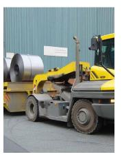
**TERMINAL TRACTORS** Pull coils on transfer carts to storage and staging areas
