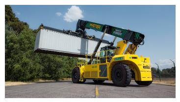
Arrived at the Port of Valencia for testing in late 2023. A hydrogen fuel cell engine converts hydrogen to electricity, offering similar laden container handling performance to diesel-powered equipment and the ability to refuel in as little as 10-15 minutes.
