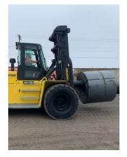
**COIL-HANDLING LIFT TRUCK** Picks coils from storage yard and transfers to loading area
