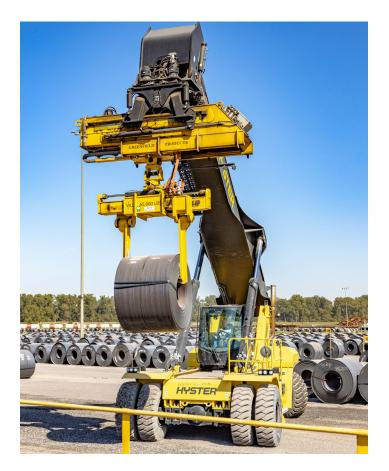
But a ReachStacker appropriately equipped for coil handling can safely and effectively execute all the coil picking, transportation and loading functions handled by fixed or moving cranes, conventional counterbalance lift trucks and ram tractors in a traditional application.
