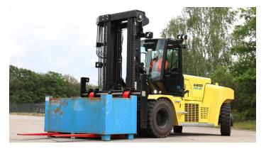
High-performance 350-volt lithium-ion battery power delivers performance comparable to traditional dieselpowered trucks for heavy-duty industries like steel, concrete, lumber, agriculture and ports.
