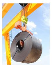
**OVERHEAD / GANTRY CRANE** Pick and load coils for shipment
