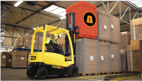
OVERLOAD ARREST to prevent lifting and carrying loads that exceed weight limits
