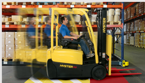
AUTOMATIC SLOWDOWN when approaching the end of an aisle or intersection
