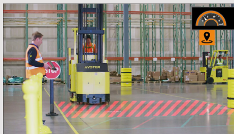
SPEED CONTROL ZONES help reduce travel speed within designated areas in the facility
