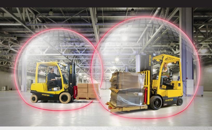
Hyster Reaction<sup>™</sup> is an industry-first technology package that helps reinforce lift truck operating best practices, tailored to the complexity of demanding, fast-paced indoor lift truck environments. The solution applies a broad range of equipment performance controls based on location, equipment-specific thresholds and proximity to obstacles or pedestrians, while the operator remains in control of the lift truck.
