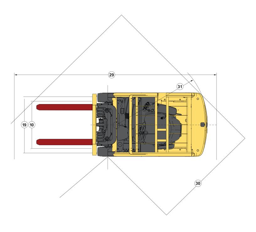
Circled dimensions correspond to the line numbers on the tabulated chart inside the technical guide. Dimensions are in inches (millimeters).
