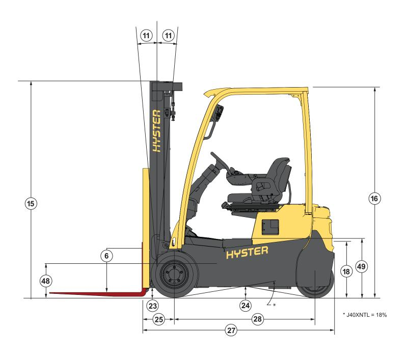
Circled dimensions correspond to the line numbers on the tabulated chart inside the technical guide. Dimensions are in inches (millimeters).
