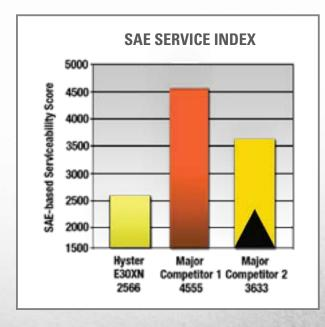
The Society of Automotive Engineers (SAE) based rating evaluating speed and difficulty of over 30 service routines. Lower score indicates easier serviceability.
