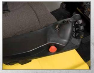
Electro-hydraulic controls with TouchPoint mini-levers
