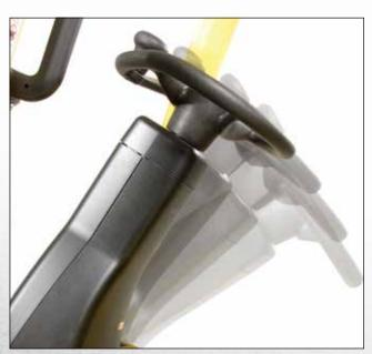
Infinitely adjustable tilt steer column
