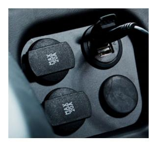
Operators can stay connected and charged with up to 2 USB Ports located in the control arm and behind the seat with an AC/DC power outlet.
