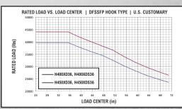
Rated capacities are for trucks equipped with: • 2-stage (lower mast) to 147" (3750 mm) maximum fork height • 105" (2672 mm) carriage width (H400XDIS36) • 116" (2940 mm) carriage width (H450XDI/36) • 96" (2440 mm) long forks Contact your dealer for other capacity information.
