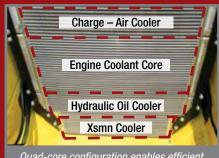
Quad-core configuration enables efficient cooling
