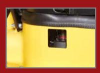
*Hydraulic sight gauge for fluid level checks*
