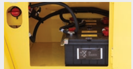
Battery compartment with lockable battery disconnect switch
