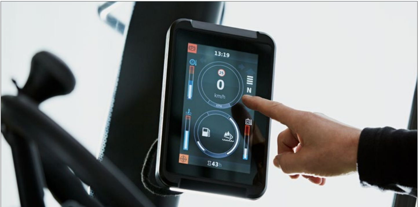
A 7 inch full-color Integrated Performance Display provides truck performance data in one clear screen.
