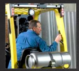
Open rearward visibility when operating in reverse. An optional rear drive handle with horn button makes reverse operation easier.
