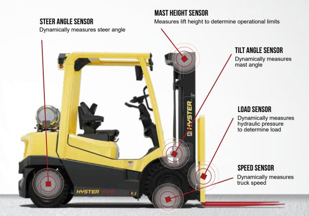
DSS actively monitors five integrated maintenance-free sensors during operation to provide information to the Vehicle System Manager (VSM). The VSM will engage DSS by providing audible and visible alerts from the operator display and limiting truck performance. If telemetry is available, the system will also send an alert to the telemetry portal.
