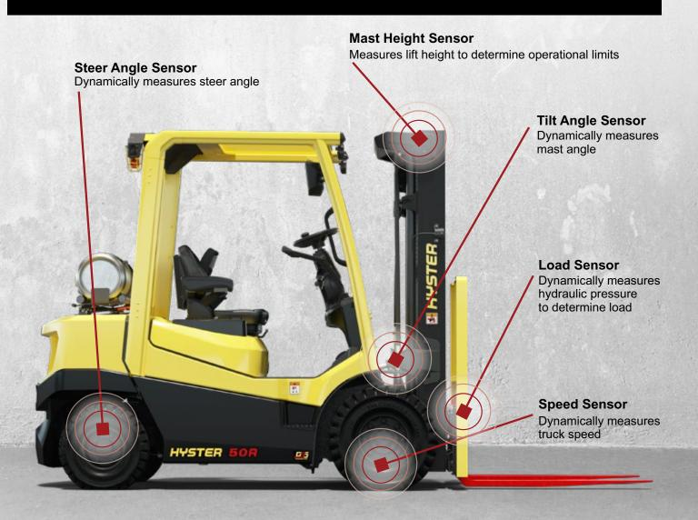
**The Dynamic Stability System (DSS)** actively monitors five integrated non-maintenance sensors during operation to provide information to the Vehicle System Manager (VSM). The VSM will engage DSS by providing audible and visible alerts from the operator display and limiting truck performance. If telemetry is available, the system will send an alert to the telemetry portal.
