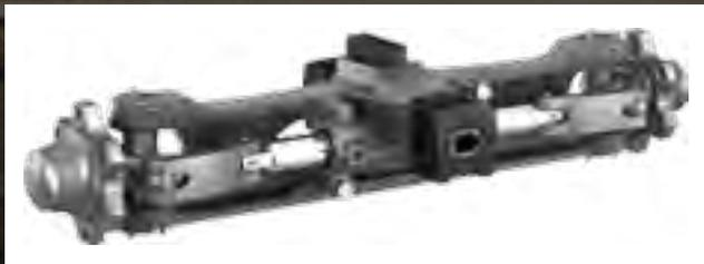
*The steer axle assembly is made of cast ductile iron. Some competitors use welded plate structures that can suffer from cracks or deformation from shock loading, or steel plate structures that can bend.*
