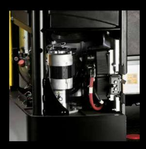
Access to the traction controller, drive motor, and hydraulic power unit is provided through the service door via a quick-release latch
