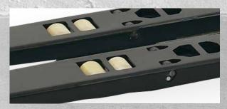
By increasing load wheel contact area, the optional tandem load wheels offer extended load wheel life under an increased load.
