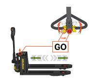
Press and hold: reverse button + forward throttle, power on
