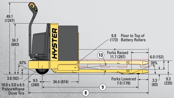
Circled dimensions correspond to the line numbers on the tabulated chart inside the Technical Guide. Dimensions are in inches (millimeters).
