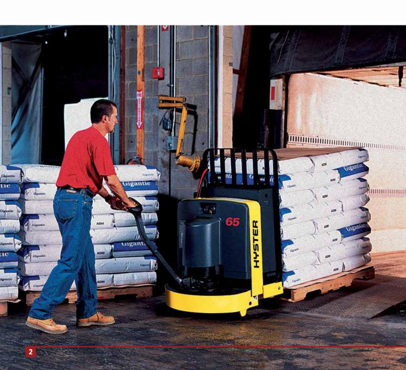
The W65Z truck's bottom-mounted handle conveniently provides you control of all functions with either hand, including the horn. Its angle hand-grips and and raised body design provide "when-you-need-it" protection for your fingers and knuckles.
