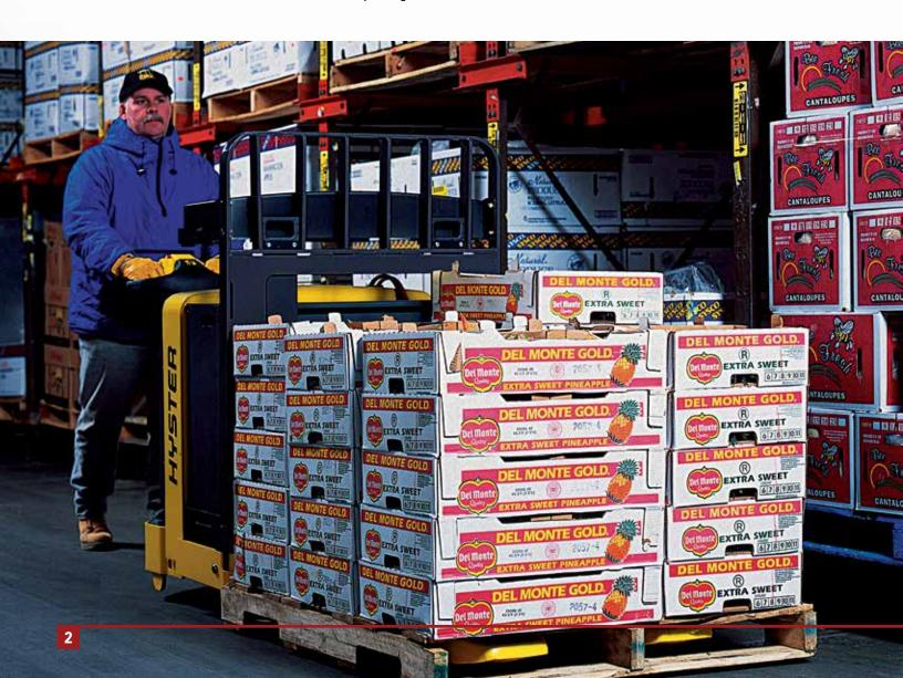
The W80Z truck's bottom-mounted handle conveniently provides you control of all functions with either hand, including the horn. Its angle hand-grips and and raised body design provide "when-you-need-it" protection for your fingers and knuckles.
